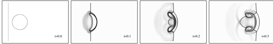
Fig. 2. Emulated Schlieren images of a shock-bubble interaction.
