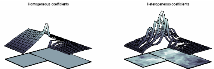
Fig. 4 -- The x-component of the velocity basis function associated with an edge/face between two blocks of different size for a homogeneous and a heterogeneous permeability field, respectively.
