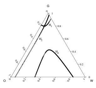
FIGURE 1. Local and detached branches of the Hugoniot loci for a reference state near the vertex of 100% gas saturation.
